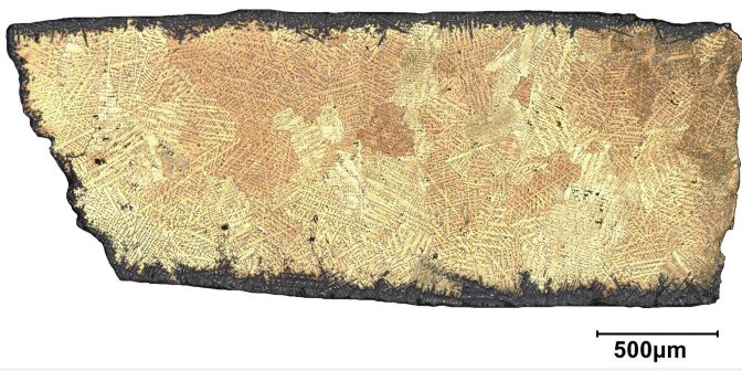
Fig. 6: Micrograph of the etched cross-section of the sample taken from the bracelet (Fig. 2) in bright field,
