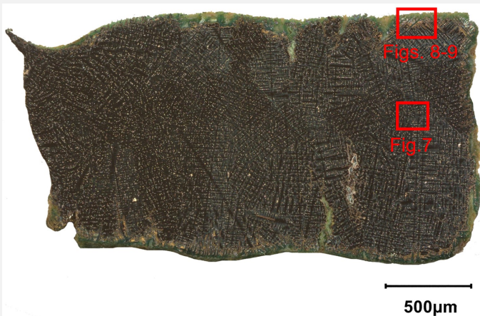
Fig. 5: Micrograph of the cross-section of the sample taken from the bracelet (Fig. 2) in dark field showing the location of Fig. 7 to 9,
