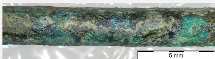
Fig. 2: Dark grey and dark green corrosion products (detail) of the pin or needle fragment near the top,
