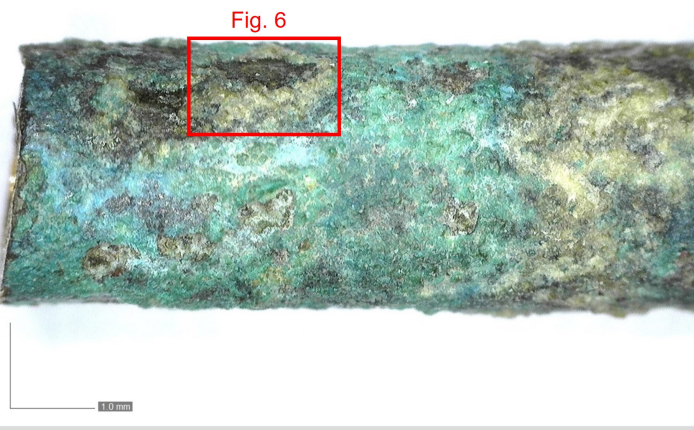
Fig. 5: Blue-green corrosion product (detail) of the pin from Fig. 4 with location of Fig. 6 (red square),
