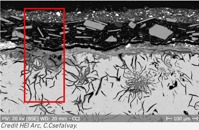
Fig. 9: SEM-image (BSE-mode) of the selected area in Fig. 8 (detail), showing the morphology of the paint layers and the area selected for elemental chemical distribution (Fig. 10) marked by a red rectangle,
