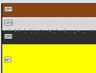
Fig. 9: Stratigraphic representation of the corrosion structure of the sickle observed macroscopically under binocular microscope using the MiCorr application with reference to Fig. 8. The characteristics of the strata, such as discontinuity, are accessible by clicking on the drawing that redirects you to the search tool by stratigraphy representation, Credit HE-Arc CR, L.Rémy.
