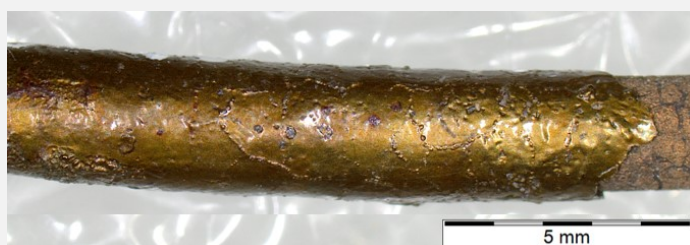
Fig. 4: Dense and smooth olive green corrosion products on the middle of the pin (detail). A grain-like structure can be seen on the surface,
