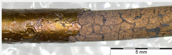
Fig. 3: Dense and smooth olive green corrosion products on the middle of the pin (detail). Discontinuity in the layer is showing the underlying corrosion structure,
