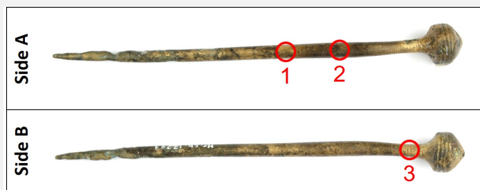
Fig. 5: Sides A and B (opposite sides) of the pin showing the XRF analysis areas (red circles),
