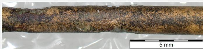
Fig. 3: Brown-yellow corrosion products (detail) on the middle part of the pin,
