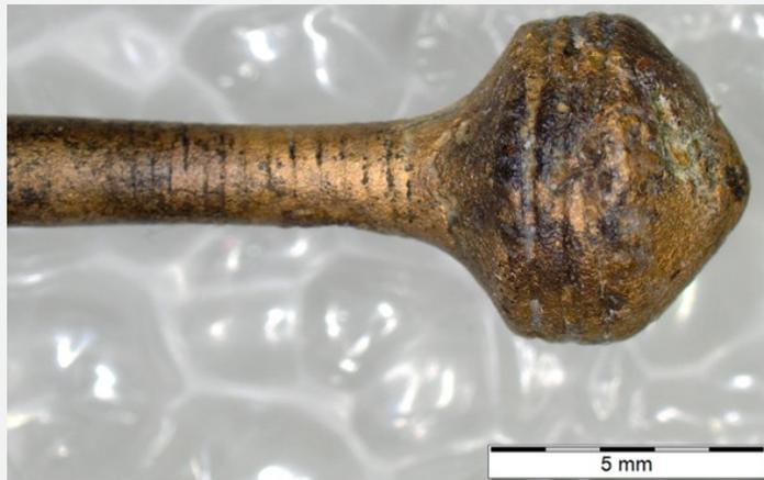
Fig. 2: Brown-yellow corrosion products (detail) around the head of the pin,
