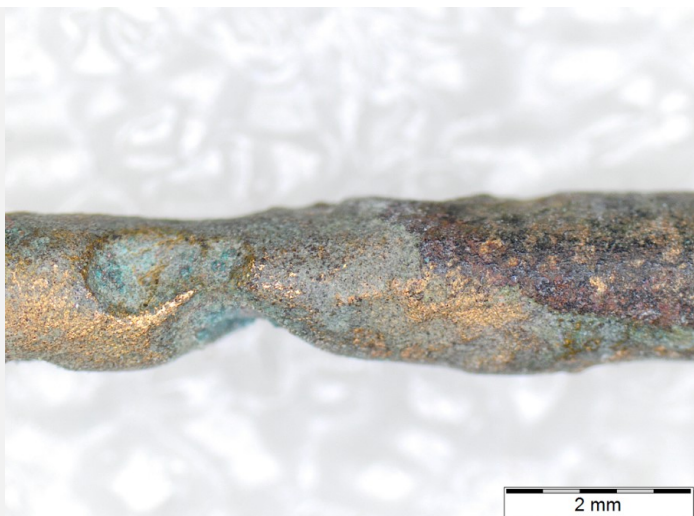
Fig. 4: Brown-yellow and green corrosion products (detail) in an area close to the tip of the pin,
