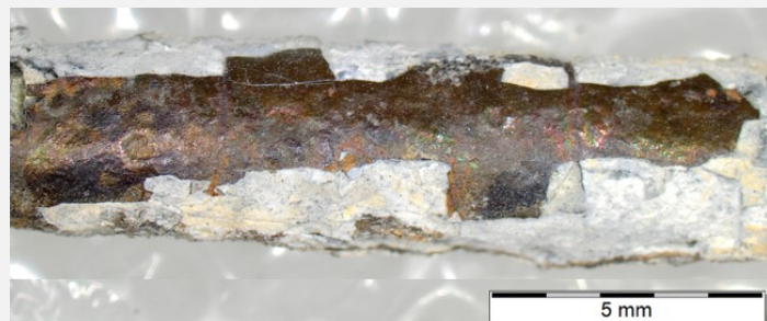
Fig. 3: White and brown corrosion products (detail) on an area in the middle of the pin,
