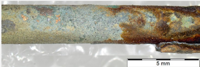
Fig. 5: Brown and green corrosion products (detail) on an area in the middle of the pin,
