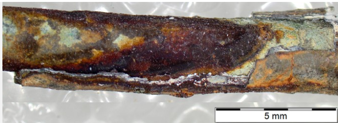
Fig. 4: White and brown corrosion products (detail) on an area in the middle of the pin,
