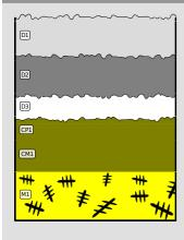
Fig. 5: Stratigraphic representation of the corrosion structure of the bracelet observed macroscopically under binocular microscope using the MiCorr application with reference to the whole Fig. 4. The characteristics of the strata are only accessible by clicking on the drawing that redirects you to the search tool by stratigraphy representation, Credit HE-Arc CR, N.Gutknecht.
