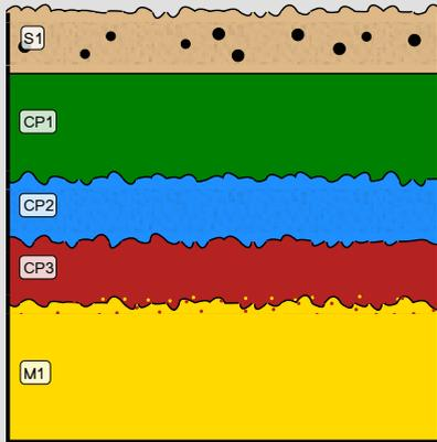
Fig. 4: Stratigraphic representation of the corrosion structure of the bracelet observed macroscopically under binocular microscope using the MiCorr application with reference to the whole Fig. 3. The characteristics of the strata are only accessible by clicking on the drawing that redirects you to the search tool by stratigraphy representation, Credit HE-Arc CR, N.Gutknecht.
