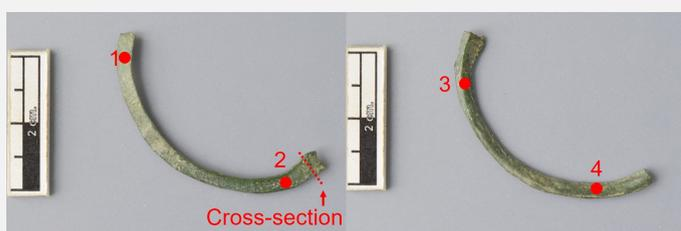
Fig. 2: Side B (left) and side A (right) of bracelet showing the sampling area and the XRF analysis areas (red dots),
