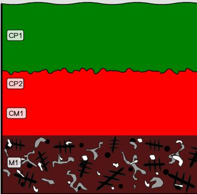
Fig. 12: Stratigraphic representation of the sample of the bracelet observed in cross-section under dark field using the MiCorr application. The characteristics of the strata are only accessible by clicking on the drawing that redirects you to the search tool by stratigraphy representation. This representation was build according to Fig. 9, Credit LMC-CNRS, V.Valbi.
