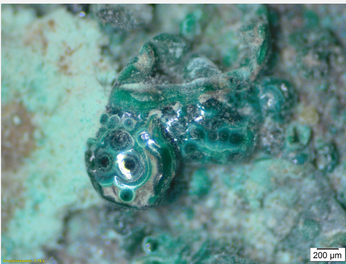
Fig. 7: Detail of Fig. 4 with green corrosion product, with eye-like structure, sample 3 (CP3)
