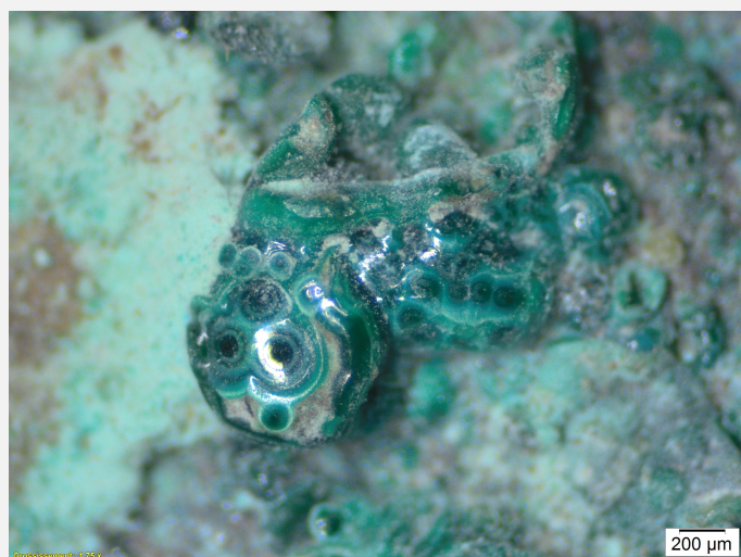
Fig. 7: Detail of Fig. 4 with green corrosion product, with eye-like structure, sample 3 (CP3)
