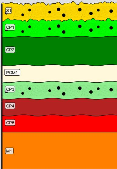
Fig. 4: Stratigraphic representation of the corrosion structure of the cooking pot handle fragment observed macroscopically under binocular microscope using the MiCorr application (to be compared to Fig. 3). The stratum SV1 is integrated in CP2 while POM1 and POM2 are merged as POM1. The characteristics of the strata are only accessible by clicking on the drawing that redirects you to the search tool by stratigraphy representation, Credit HE-Arc CR, L.Ruynat.
