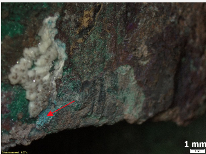
Fig. 17: Observation of the light blue corrosion product,
