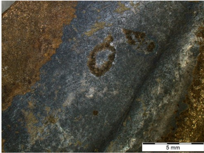
Fig. 3: Brown-yellow and dark-grey corrosion products (detail) of an area close to the tip of the sickle,
