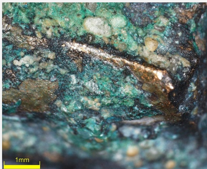
Fig. 2: Shiny yellow and green-blue corrosion products on the surface of the tang fragment of a knife.
