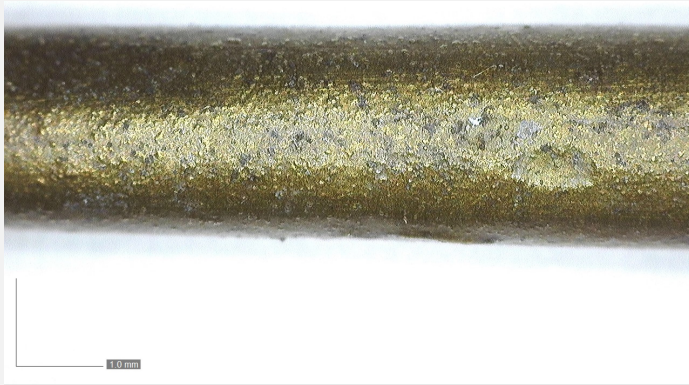
Fig. 2: Dense and smooth brown-yellow corrosion product (detail) of the pin,
