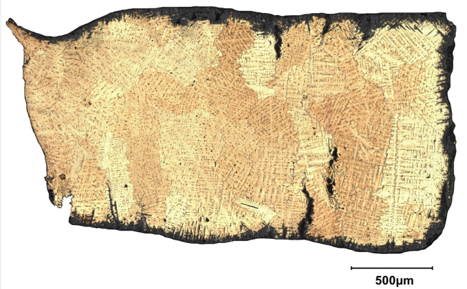
Fig. 6: Micrograph of the etched cross-section of the sample taken from the bracelet (Fig. 2) in bright field,
