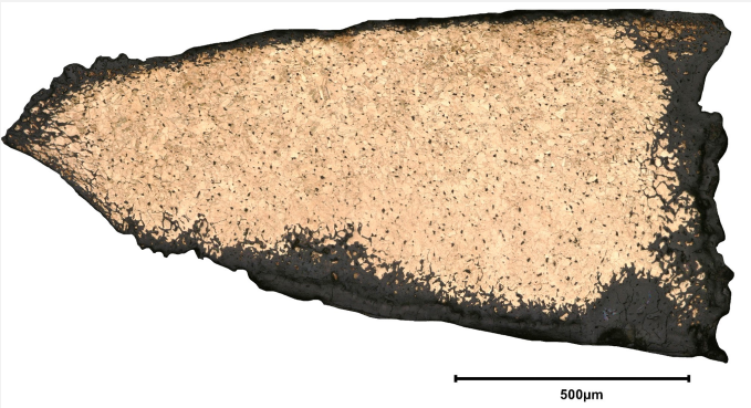
Fig. 6: Micrograph of the etched cross-section of the sample taken from the bracelet (Fig. 2) in bright field,
