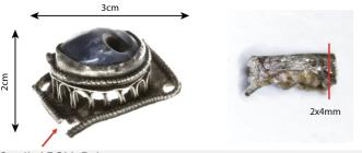
Fig. 5: Location of the analyzed tarnished fragment of setting Cv44.02 and of the sampling area. Assembly by solder between the bottom plate and the twisted wire. Dimensions:  $4 \times 2$  mm,
