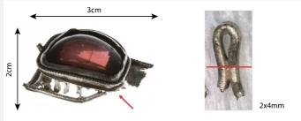
Fig. 3: Location of the analyzed fragments (3) of setting Bv35.02 and of the sampling area on the arcature tarnished fragment soldered on itself. Dimensions:  $4 \times 2$  mm,
