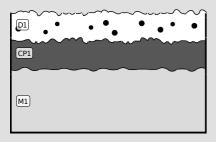
Fig.7: Stratigraphic representation of the corrosion structures of the Bv35.02, Bv49.07 & Cv44.02 settings observed macroscopically under binocular microscope using the MiCorr application with reference to Fig. 6. The characteristics of the strata are only accessible by clicking on the drawing that redirects you to the search tool by stratigraphy representation. Credit HE-Arc CR, N. Gutknecht.
