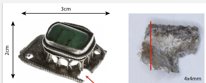
Fig. 4: Location of the analyzed tarnished fragment covered with deposits of cleaning products of setting Bv49.07 and of the sampling area. Assembly by solder between the bottom plate and the twisted wire. Dimensions: 4 x 4 mm,
