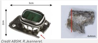
Fig. 4: Location of the analyzed tarnished fragment covered with deposits of cleaning products of setting Bv49.07 and of the sampling area. Assembly by solder between the bottom plate and the twisted wire. Dimensions:  $4 \times 4$  mm,
