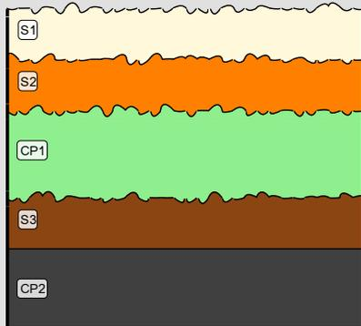
Fig. 7: Stratigraphic representation of the corrosion structure of the bust observed macroscopically under binocular microscope using the MiCorr application. The characteristics of the strata are only accessible by clicking on the drawing that redirects you to the search tool by stratigraphy representation. This representation can be compared to Fig. 5, Credit HE-Arc CR, C.Degrigny.
