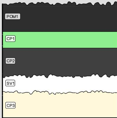
Fig. 6: Stratigraphic representation of the corrosion structure of the bust observed macroscopically under binocular microscope using the MiCorr application. The characteristics of the strata are only accessible by clicking on the drawing that redirects you to the search tool by stratigraphy representation. This representation can be compared to Fig. 5, Credit HE-Arc CR, C.Degrigny.
