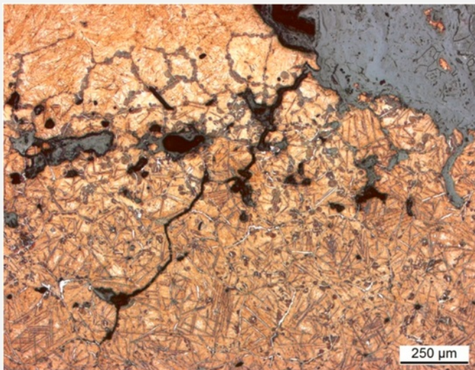
Fig. 5: Micrograph of the metal sample, detail from Fig. 4, etched, bright field. We observe martensite (in orange), cementite (in grey), porosity and intergranular cracks (in black) and corrosion,
