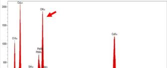
Fig. 13: EDS analysis of the green corrosion powder (Fig. 2). Method of analysis: SEM-EDS, Lab of Electronic Microscopy and Microanalysis, IMA (Néode), HEI Arc,
