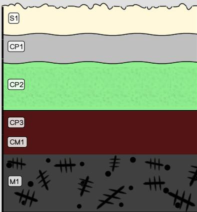
Fig. 15: Stratigraphic representation of sample from Fig. 2 of the headrest (or horse bit) in cross-section (dark field) using the MiCorr application. The characteristics of the strata are only accessible by clicking on the drawing that redirects you to the search tool by stratigraphy representation. This representation can be compared to Fig 10, Credit HE-Arc CR.
