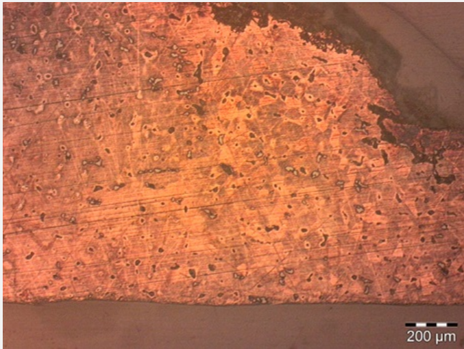
Fig. 7: Micrograph of the metal sample from Fig. 4 showing a dendritic structure and grains,
