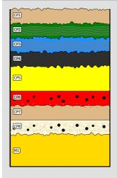
Fig. 6: Stratigraphic representation of the corrosion structure of the tang observed macroscopically under binocular microscope using the MiCorr application with reference to the whole Fig. 5. The characteristics of the strata, such as discontinuity, are accessible by clicking on the drawing that redirects you to the search tool by stratigraphy representation, Credit HE-Arc CR, N.Gutknecht,
