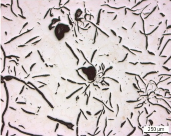
Fig. 4: Micrograph of the metal sample from Fig. 3 (inverted picture, detail), unetched, bright field. We observe graphite flakes and irregular nodules in black and the metal in white. The small grey spots are manganese sulphide inclusions,
