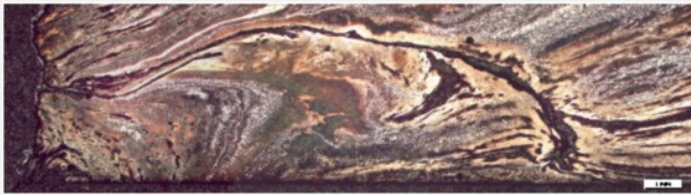
Fig. 5: Micrograph of the metal sample from Fig. 3 (reversed picture, detail), etched with Oberhoffer's reagent, bright field. The etching shows the P segregation near the welding line and outlines the irregular P distribution in the metal (white P-rich areas, dark P-poor areas),
