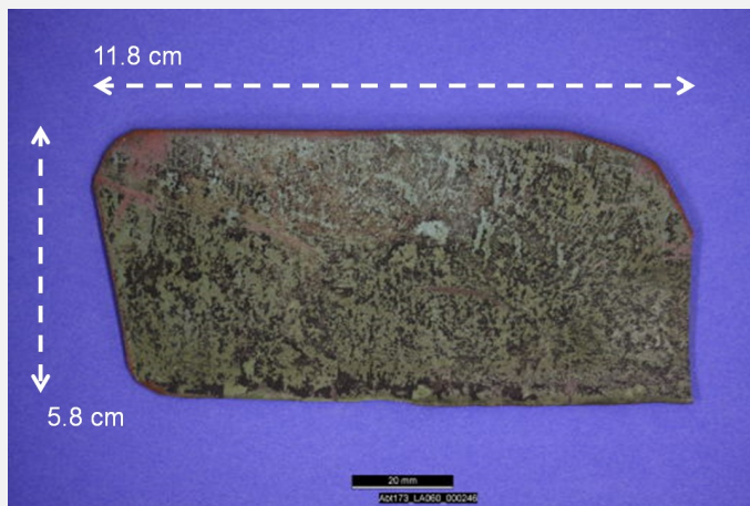
Fig. 1: Shingle of a roof, internal side,
