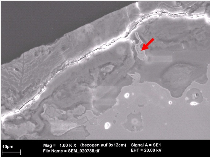
Fig. 6: SEM image of the metal sample (detail of Fig. 4, reversed picture), SE-mode. From bottom right to top left: the metal, the inner and outer corrosion layers separated by a large fissure. The red arrow indicates a remnant of the Sn-rich alpha-delta eutectoid,
