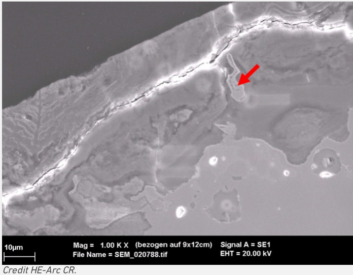
Fig. 6: SEM image of the metal sample (detail of Fig. 4, reversed picture), SE-mode. From bottom right to top left: the metal, the inner and outer corrosion layers separated by a large fissure. The red arrow indicates a remnant of the Sn-rich alpha-delta eutectoid,
