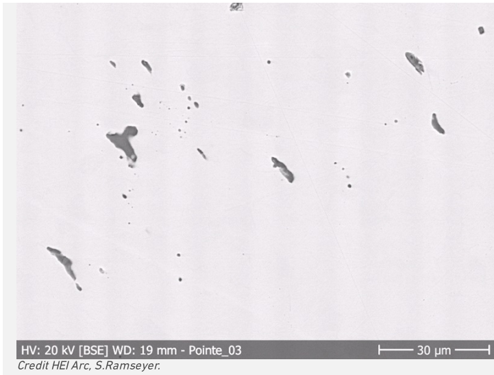
Fig. 6: SEM, BSE-mode picture of inclusions in remaining metal (detail of Fig. 5),
