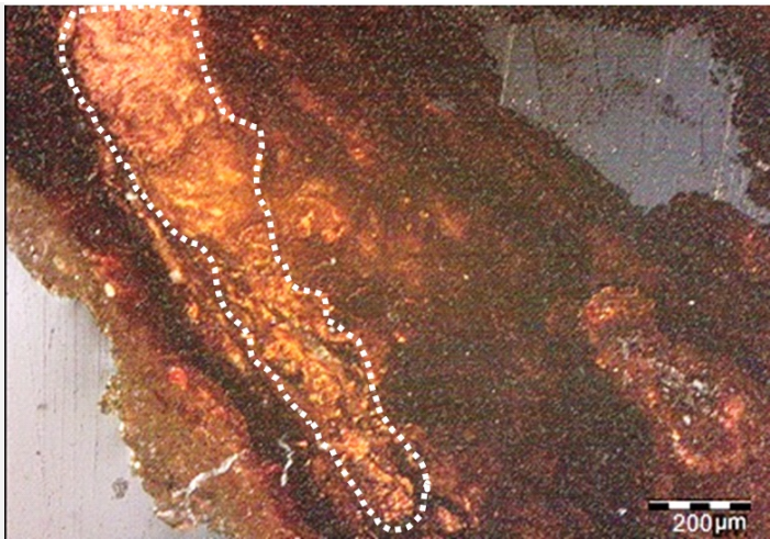
Fig. 9: Micrograph of the metal sample from Fig. 4, bright field. The delimited zone shows what could be leather pseudomorphic fibers filling a void,
