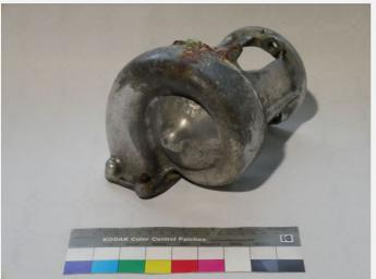
Fig. 1: Hispano-suiza water pump, unknown model,
