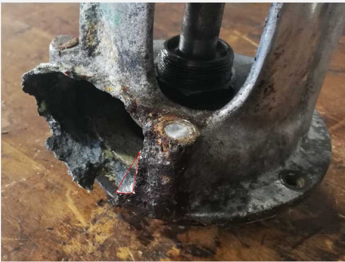
Fig. 5: Close-up view of the corroded exit pipe of the disassembled Hispano water pump, showing the sampled area,
