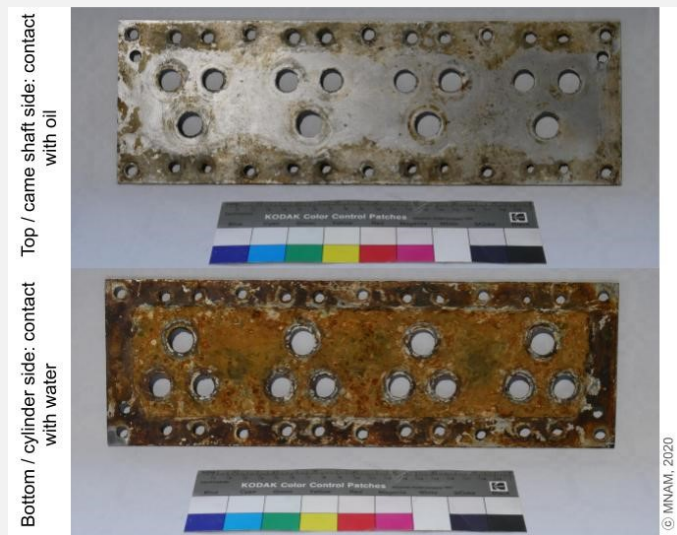
Fig. 1: General picture of the corroded cylinder head gasket of the Bugatti Type 37. Top side facing the camshaft and bottom part in contact with the coolant of the block,
