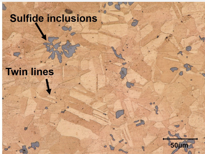
Fig. 8: Micrograph of the metal sample from Fig. 7 (detail), etched, bright field. In color, polygonal grains with twin lines and in grey sulfide inclusions,
