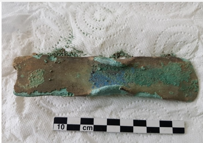
Fig. 1: Winged axe covered with a brown crust and blue-green corrosion products and showing areas of flaking,
