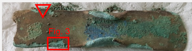
Fig. 2: Axe with location of Fig.3 and sampling area (red triangle),
