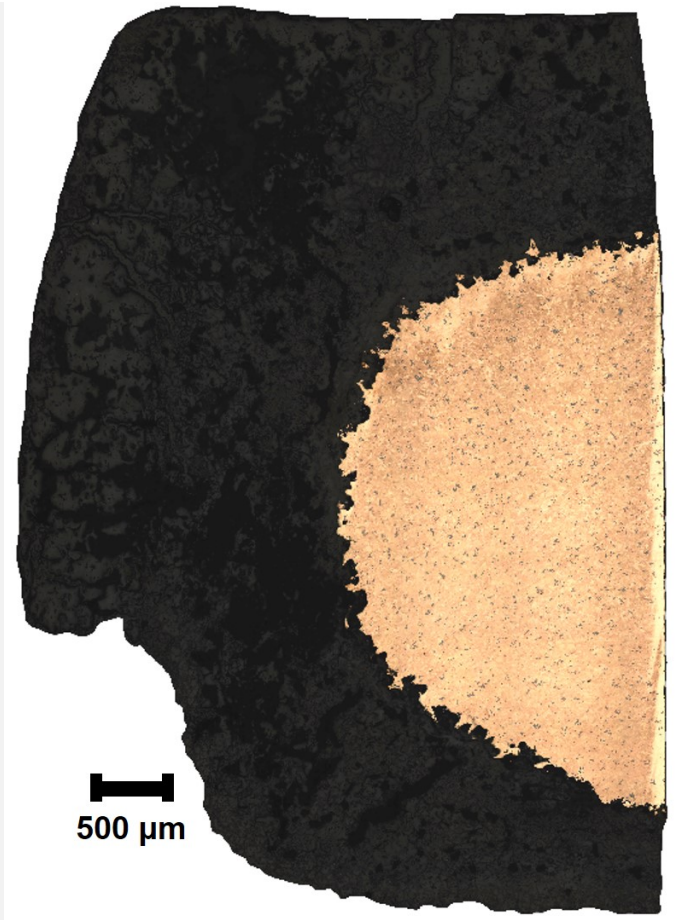
Fig. 7: Micrograph of the cross-section of the sample (same as Fig. 6) in bright field after chemical etching,
