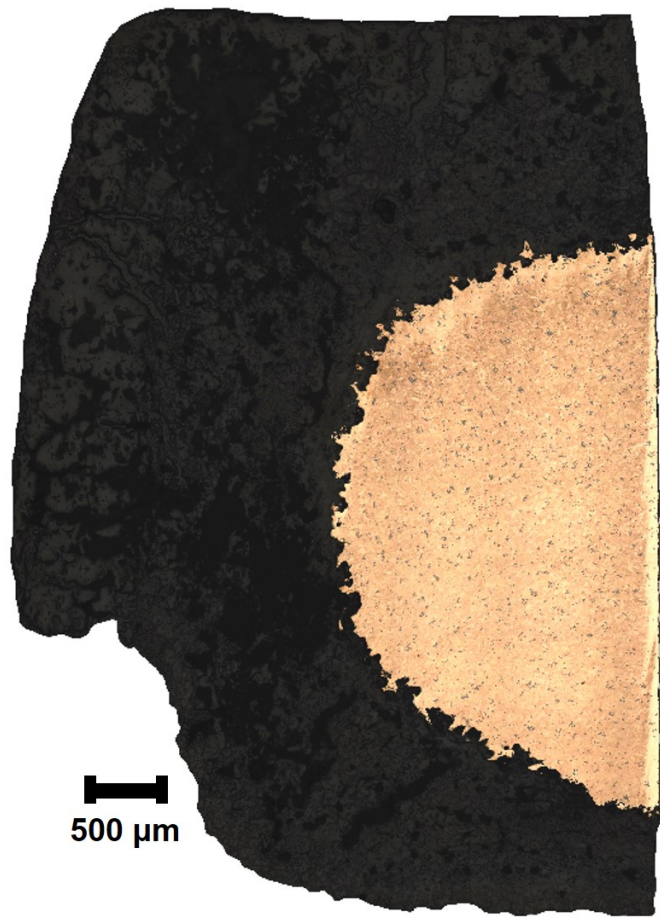
Fig. 7: Micrograph of the cross-section of the sample (same as Fig. 6) in bright field after chemical etching,
