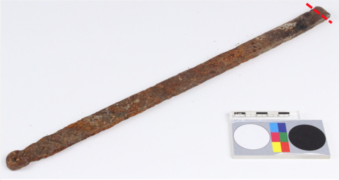
Fig. 2: Location of sampling area (a cross-section of the metal, marked by a stippled line),
