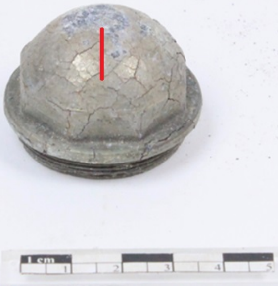
Fig. 2: Zone of the artefact submitted to visual observation and location of sampling area (a cross-section of the metal marked by the red line),
