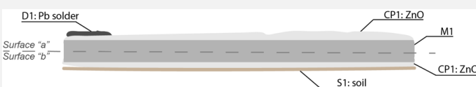
Fig. 15: Improved stratigraphic representation of the roof gutter element with results from analyses by SEM-EDS, XRD and visual microscopic observation. CP = corrosion product, D = deposit, M = metal, S = soil,
