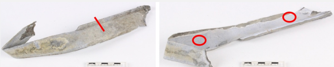
Fig. 2: Location of sampling area (a cross-section through the metal marked by the stippled line) and of powder samples (red circles),
