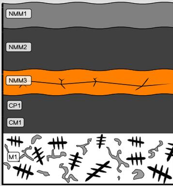
Fig. 11: Stratigraphic representation of the sample taken from the lamp post (?) fragment in cross-section (dark field) using the MiCorr application. The characteristics of the strata are only accessible by clicking on the drawing that redirects you to the search tool by stratigraphy representation. This representation can be compared to Fig. 8, Credit UiO-IAKH, M.Hovind.
