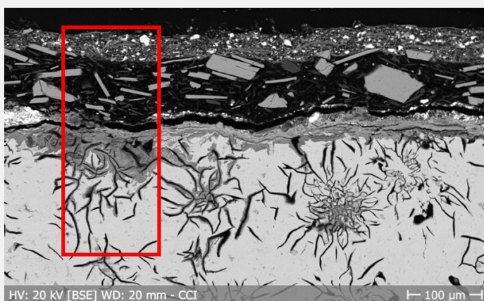
Fig. 9: SEM-image (BSE-mode) of the selected area in Fig. 8 (detail), showing the morphology of the paint layers and the area selected for elemental chemical distribution (Fig. 10) marked by a red rectangle,
