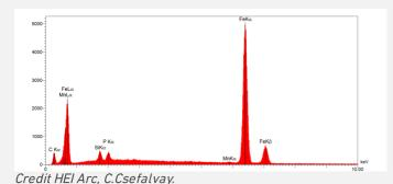
Fig. 5: EDS-spectrum showing the chemical composition of the metal. Method of analysis: SEM-EDS. Lab. of Electronic Microscopy and Microanalysis, Néode, HEI Arc,
