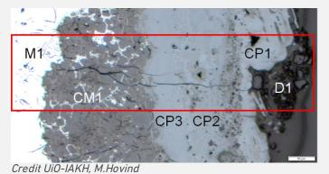
Fig. 7: Micrograph of the metal sample from Fig. 4 (detail), unetched, polarized light, 5x. Stratigraphy of the exterior surface, to be compared to Fig. 11 and from top to bottom: the metal (M1) in grey, a layer of corroded metal (CM1) followed by a thin layer of CP1, and a white cracked layer (NMM1) superimposed by a porous dark-red deposit (D1),
