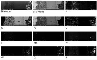
Fig. 10: SEM image and elemental chemical distribution of the selected area from Fig. 8. Method of analysis: SEM-EDS. Lab. of Electronic Microscopy and Microanalysis, Néode, HEI  $\Delta rc$
