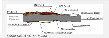
Fig. 13: Improved stratigraphic representation of the rain gutter fragment based on analysis from cross-section and visual microscopic observation,
