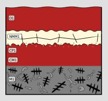
Fig. 11: Stratigraphic representation of the sample taken from the rain gutter fragment in cross-section (dark field) using the MiCorr application. The characteristics of the strata are only accessible by clicking on the drawing that redirects you to the search tool by stratigraphy representation. This representation can be compared to Fig. 7 (exterior surface). CP1 corresponds to CP2 in Fig. 3, Credit UiO-IAKH, M.Hovind.
