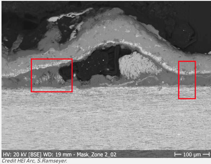
Fig. 6: SEM image (BSE-mode) of the metal sample from Fig. 4 with detail (Fig. 7) indicated by the left red rectangle. The selected area for elemental chemical distribution (Fig. 8) is marked by the right red rectangle,
