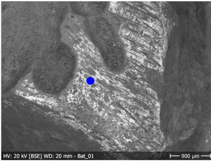
Figs. 8: SEM images of the metal on the nose of the bat. The blue point represents the area for the EDS point analysis (Fig. 9),
