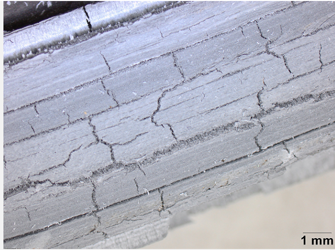
Fig. 3: Detail of the corroded lead came,
