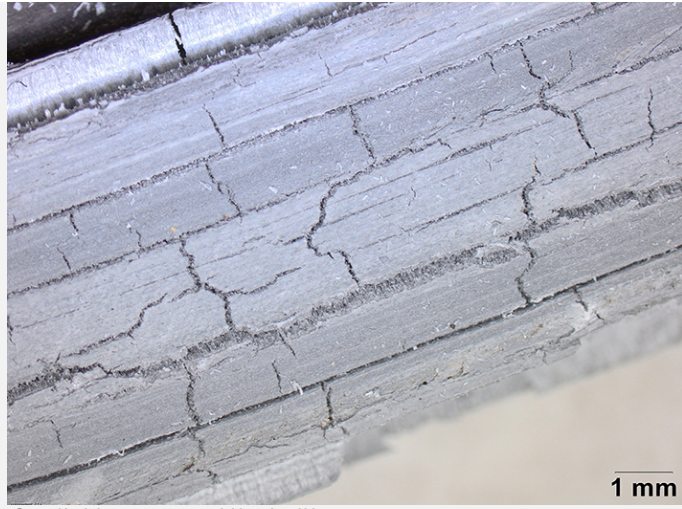
Fig. 3: Detail of the corroded lead came,
