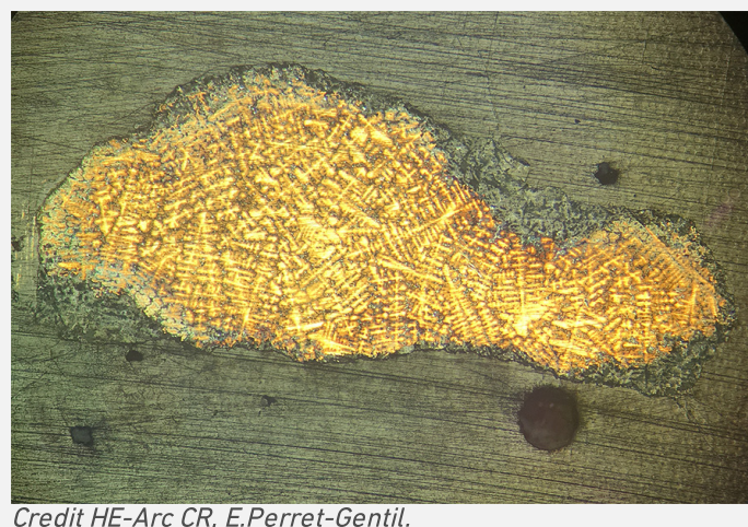
Fig. 13 : Micrograph showing the dendritic microstructure (reversed picture of Fig. 12), etched, bright field,
