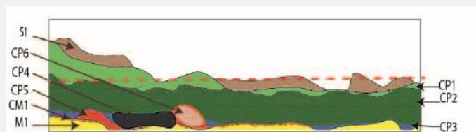
Fig 22 : Improved representation of the stratigraphy of corrosion layers of the bracelet from visual observations and analyses,
