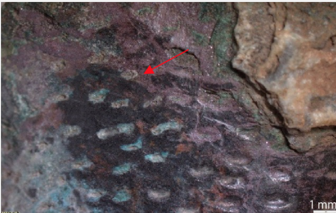
Fig. 19: Observation of the red corrosion product above the black original surface containing corresponding markers such as engravings,
