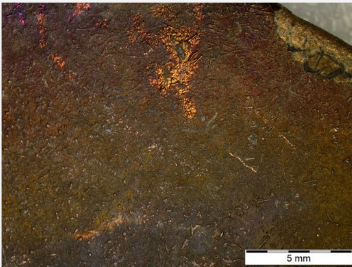
Fig. 4: Brown-yellow and dark-grey corrosion products (detail) of the middle of the sickle,
