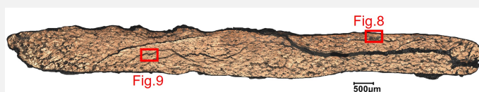
Fig. 7: Micrograph (similar to Fig. 6) of the cross-section of the sample taken from the coin (Fig. 2) in bright field after chemical etching,
