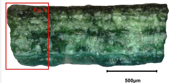
Fig. 5: Micrograph of the cross-section of the fragment from the pin (Fig. 2, left fragment) in dark field showing the location of Fig. 6. The external surface is on top,
