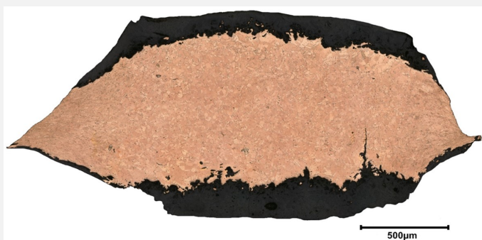
Fig. 7: Micrograph of the etched cross-section of the sample taken from the bracelet (Fig. 2) in bright field,
